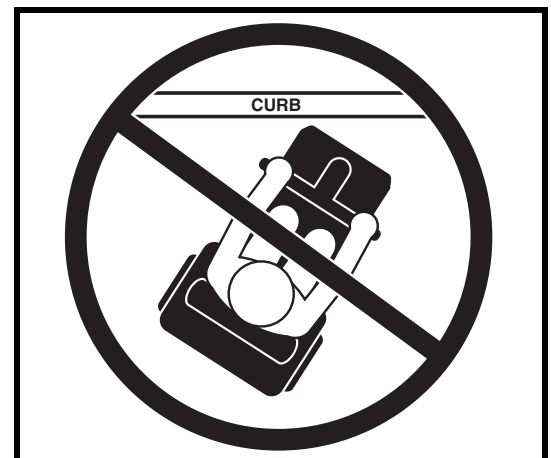
Figure 7. Incorrect Curb Approach
